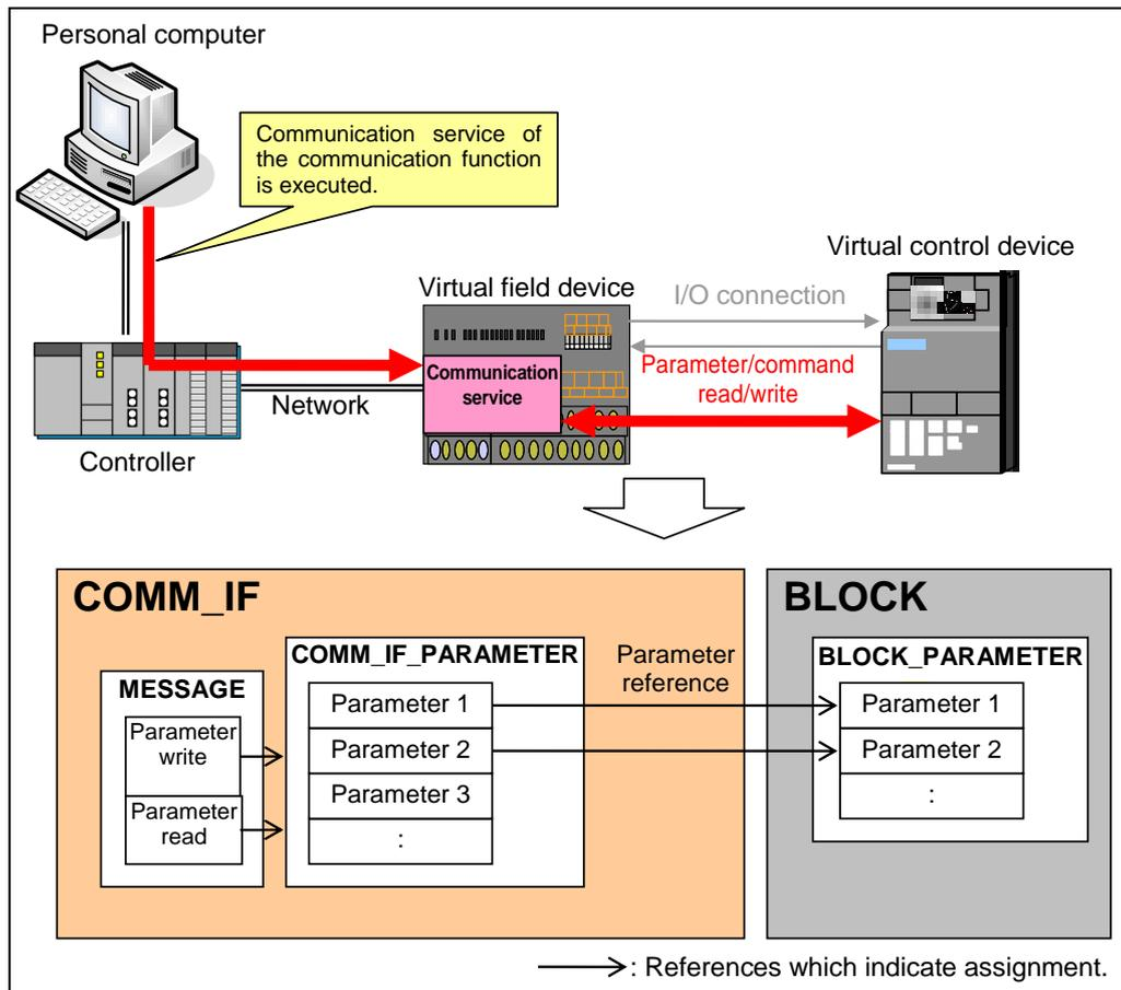
Figure 4.4-1 Reference Specifications Example of the COMM\_IF\_PARAMETER Part
