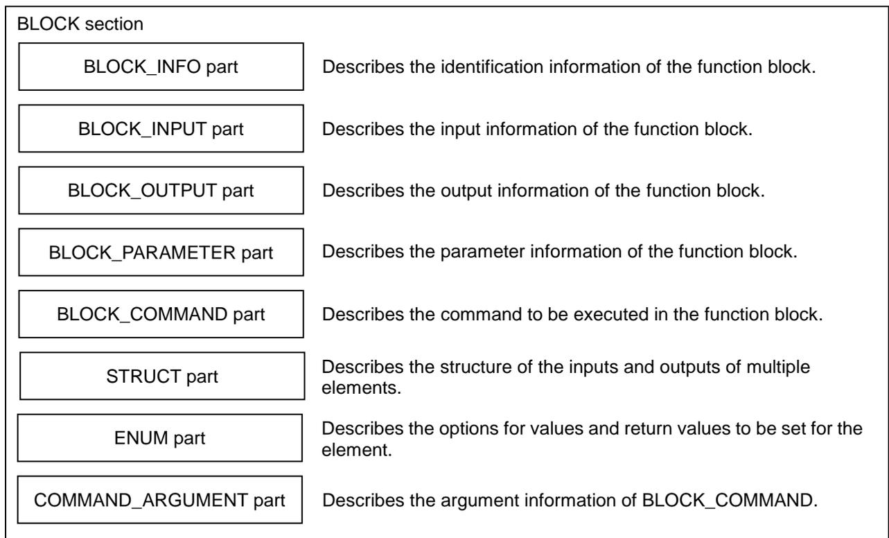
Figure 5-1 Structure of the BLOCK Section
