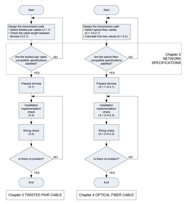
Figure 1.1-1 Installation procedure
