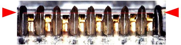
Figure A-1-3 Example of uneven pin terminal height of crimp type RJ45 connector (plug)
