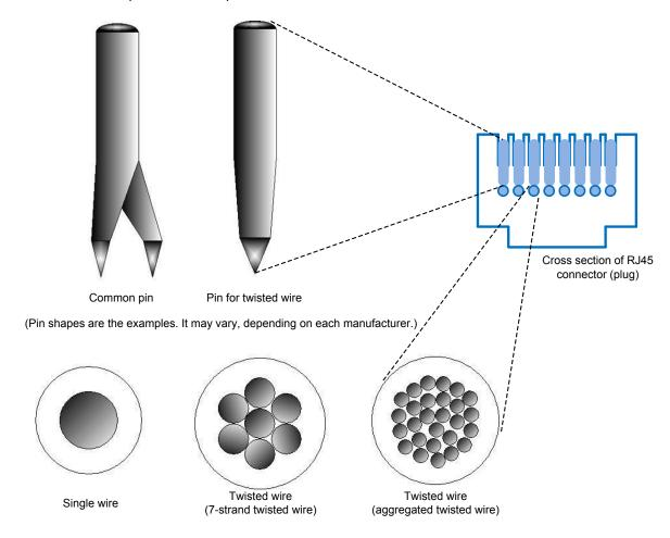
Figure A-1-1 Example pin shapes and conductor types of J45 connectors (plugs)
