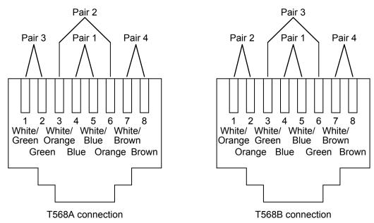
Figure 3.2-3 Connection to RJ45 Connector (Plug)
