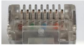
Example of normal connector Figure A-1-4 RJ45 Connector deformation cases
