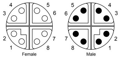
Figure 3.2-4 M12 (X-coding) connector
