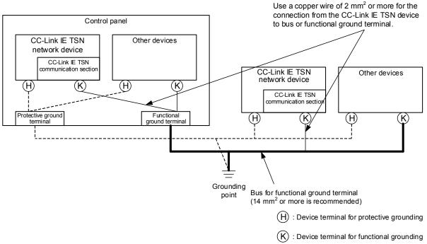
Figure 3.3-6 Wiring example of common grounding
