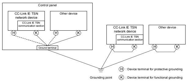
Figure 3.3-5 Example of Common Grounding
