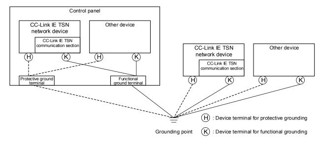
Figure 3.3-4 Example of Common Grounding
