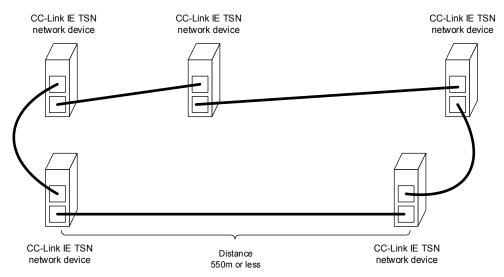
Figure 4.1.2-1 Wiring length
