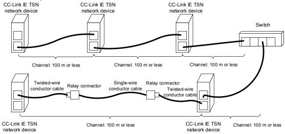
Figure 3.2-1 Wiring length
